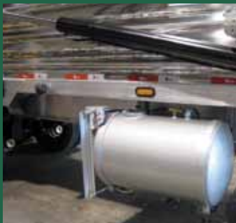
LARGE CAPACITY, PRESSURIZED WATER TANK AND HOSE
